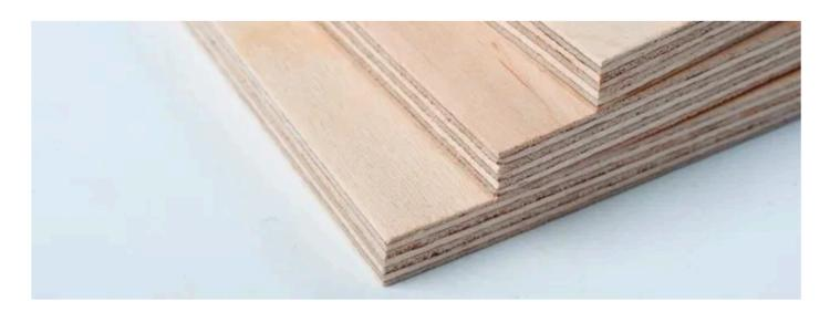
The plywood is a semi-finished wood, made of veneer sheets superimposed perpendicularly sheet by sheet, glued under pressure. With a wide specification, plywood has a wide range of uses, such as furniture, packaging, interior design, construction, etc.
