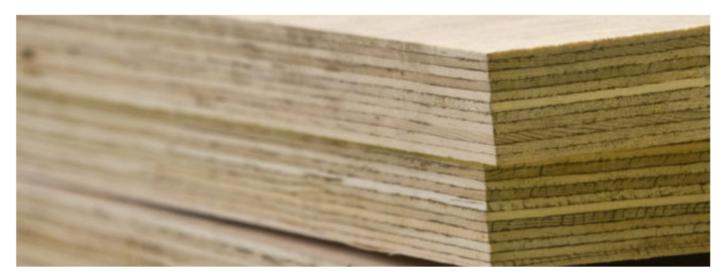
Laminated veneer lumber (LVL) is a product made of 7 or more veneer sheets of about 3 mm thick, glued at high temperature, forming a thick panel with a high degree of strength, and can be used both in the furniture industry (stairs, doors, windows, sofas), as well as in constructions (floors, roof, beams, etc.).
