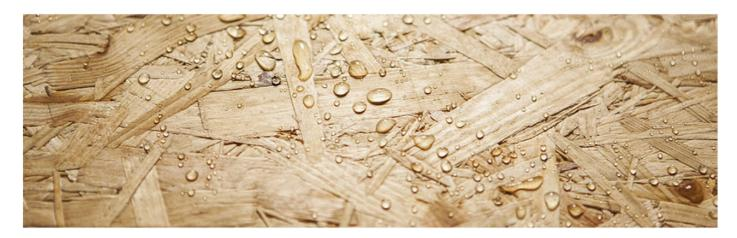
Oriented Strand Board (OSB) boards are layered wood panels made of long, thin, oriented wood chips that are glued together with a synthetic resin. The chips are pressed together in layers, the faces having chips of about 100 mm long oriented longitudinally, the core having chips arranged perpendicularly, with a length between 5 - 50 mm. Commonly used types of resins include binders that give moisture resistance to OSB panels.
