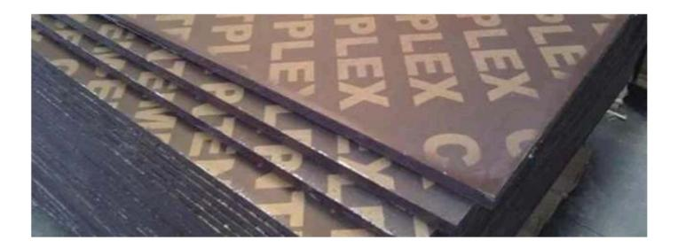
Used in formwork construction, filmed plywood is a product made of veneer sheets glued with special adhesive to withstand a high humidity environment, having applied on both sides of the phenolic film film.
